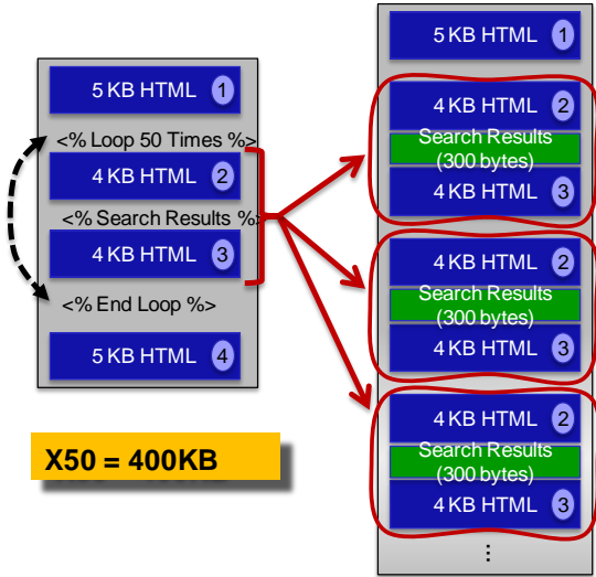
Figure 2 - Both static and dynamic data are returned with each result causing overhead
